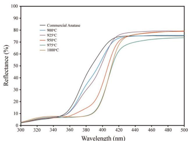
Fig. 5. The reflection spectra of the commercial anatase and annealed TiO<sub>2</sub> powders as a function of annealing temperature.
