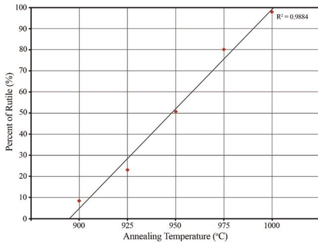
Fig. 2. Percentage of rutile phase as a function of annealing temperatures.
