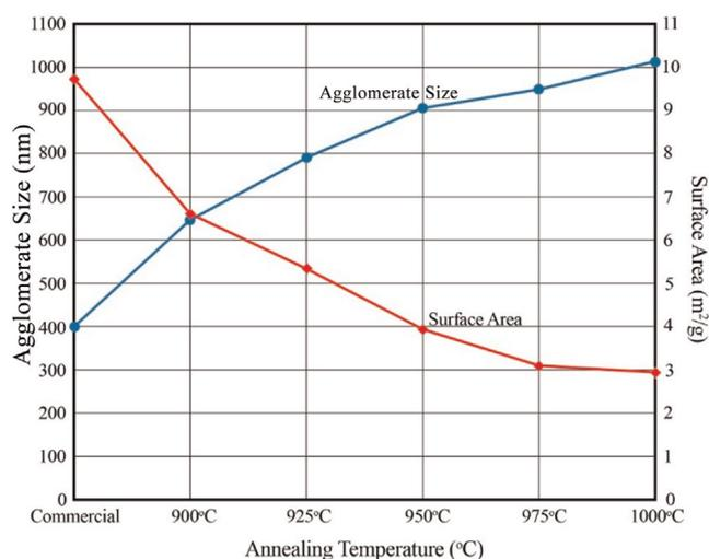
Fig. 4. The agglomerate size and specific surface area of the commercial anatase and annealed TiO<sub>2</sub> powders as a function of annealing temperature.
