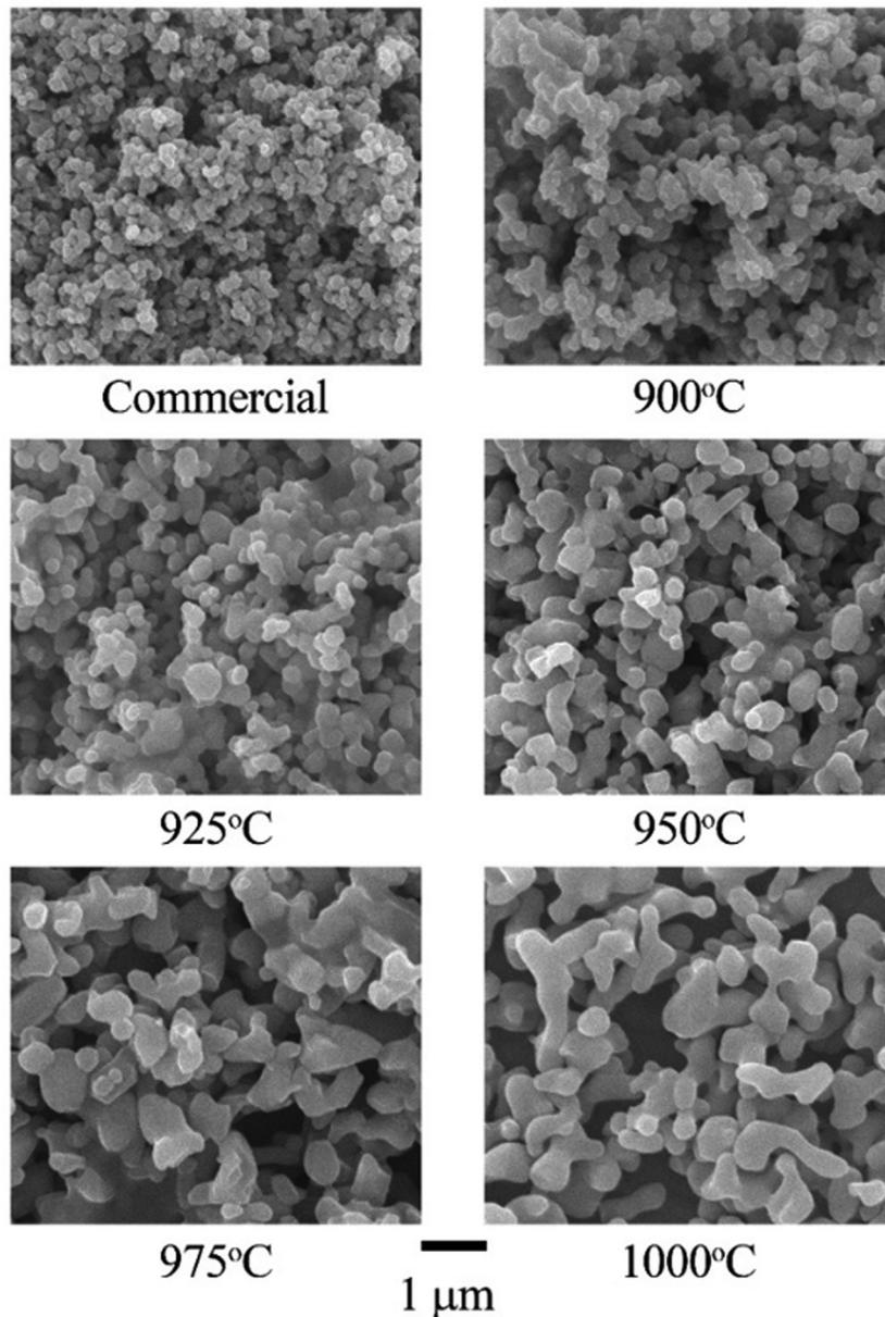
Fig. 3. SEM images of the commercial anatase and annealed  $\text{TiO}_2$  powders at different temperatures.
