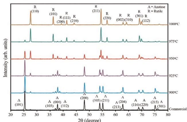
**Fig. 1.** XRD patterns of the commercial anatase and annealed  $\text{TiO}_2$  powders at different temperatures.
