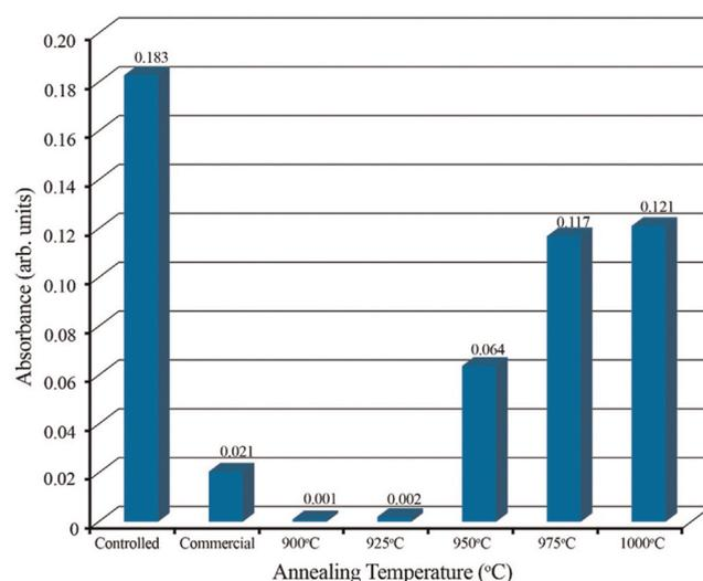
Fig. 6. MB removal performance of the commercial anatase and annealed TiO<sub>2</sub> powders at different temperatures.
