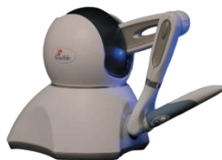
Figure 1 An example of commercial haptic device (PHANToM Omni) developed by SensAble Technologies [5]
