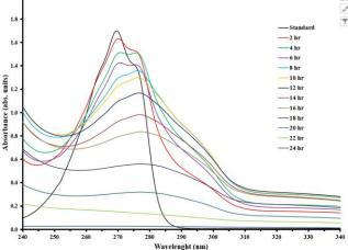
Fig. 4. The absorption spectrum of phenol at various illumination time.
