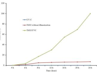
Fig. 2. Degradation of phenol under different conditions.
