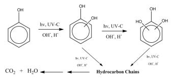
Fig. 5. The possible degradation mechanism of phenol in photocatalysis.
