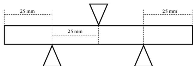
**Figure 1.** The loading geometry of 3-point bending
