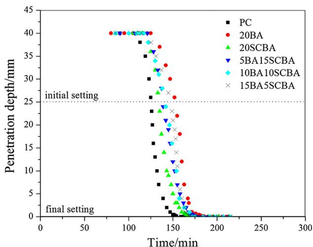
**Fig. 2** Setting time of ordinary Portland cement containing BA and SCBA
