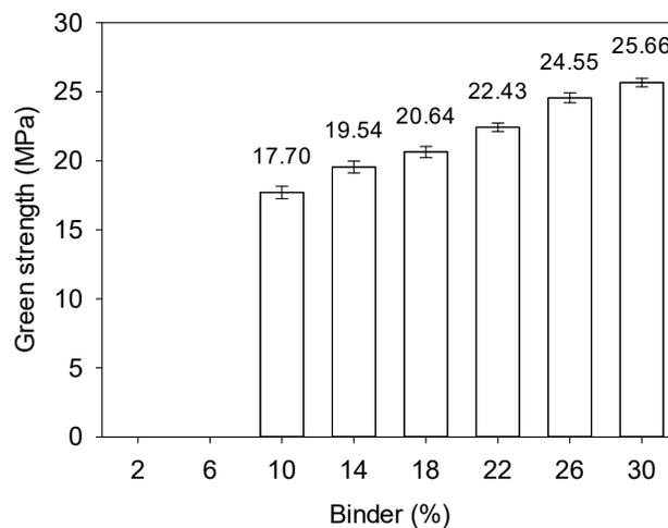
**Figure 6** Green strength from three-point bending test.
