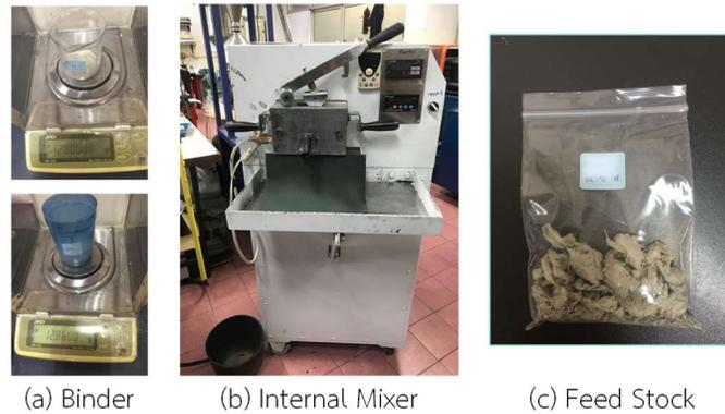
**Figure 1** Mixing process.
